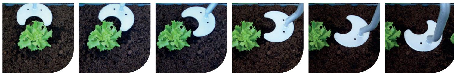
Disc profile and synchronisation setup is designed to maximise cultivated area and provide adequate tolerance to plant misalignment, in order to minimise crop damage. The tolerance required depends on the growth habit of the crop plants. For crops with regular growth habits the uncultivated area can be very small. 80mm D uncultivated plant zone is common.
